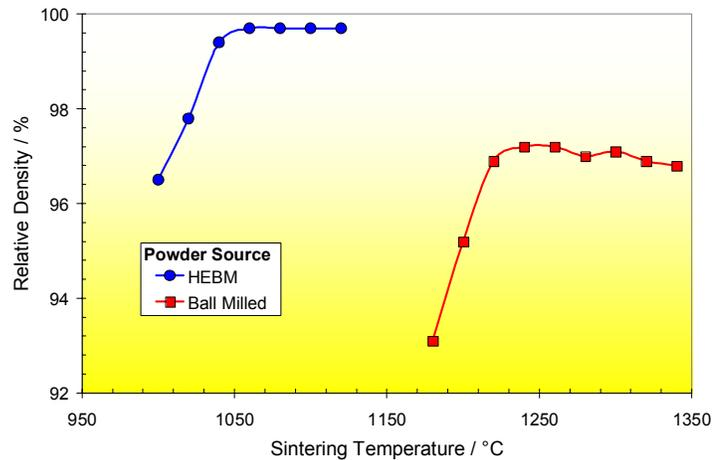
Figure 2. Relative density as a function of sintering temperature for PMNT (10mol% Ti) produced by ball millina (24 hr) and HEBM (20 mins).
