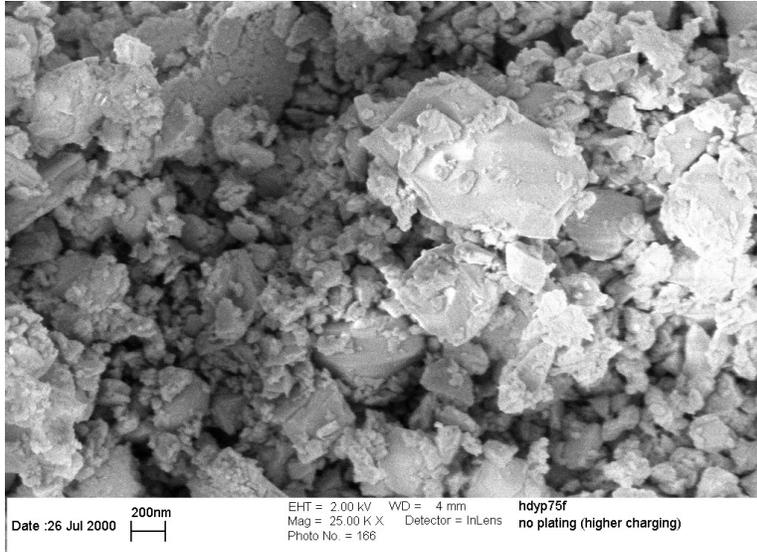
**Figure 3. Scanning Electron Micrograph of an Ecertec Ultra-Active PMNT agglomerated powder - produced using the HEBM process.**
