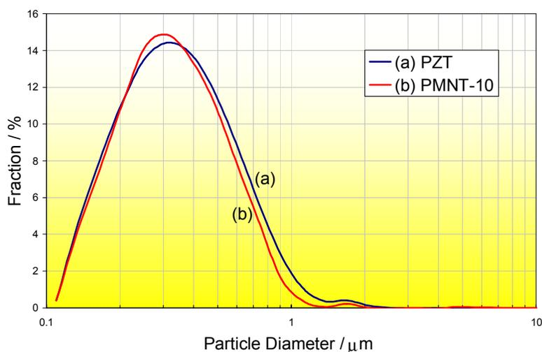
**Figure 1. Particle size distributions for Ecertec Ultra-Active HEBM powders: (a) piezoelectric PZT and (b) electrostrictive PMNT (PMN-10mol% Ti)**
